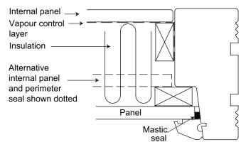
Figure 2.24: Infill panel with exposed framing
