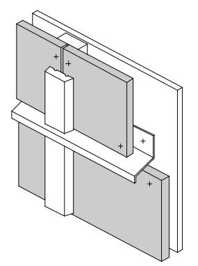
Figure 2.23: Vertical joint with timber cover battens and horizontal joint with preformed metal flashing
