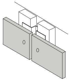
Figure 2.22: Open vertical joint with preformed metal 'top hat' flashing
