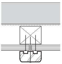
Figure 2.21: Board cladding with vertical battened joints
